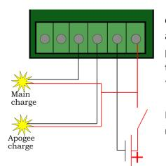
The Raven3 has a slightly-unexpected system for connecting ejection charges, as shown in the wiring diagram at left. One side of each ejection charge is wired to the positive terminal of the battery and the other end goes to the deployment channel. The Raven3 holds each channel "high" then pulls it "low" (i.e. to ground) to fire a charge.
