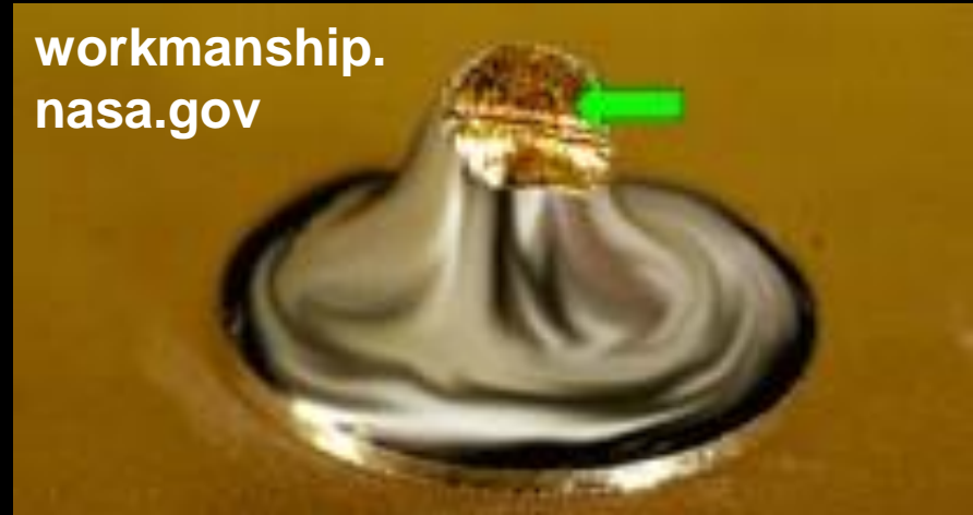
Example of a good solder filet
