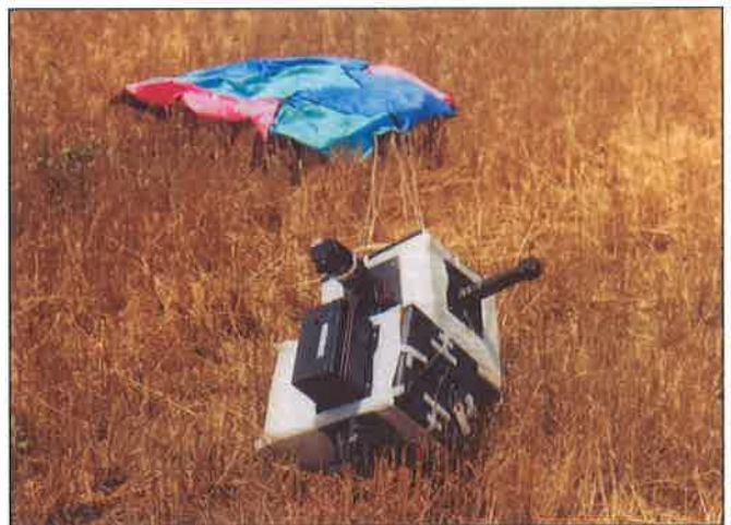
A beautiful sight — a spacecraft after its mission. APRS reports the landing position to within 100 feet. Recovery crews only had to follow their GPS receivers until the parachute was sighted.
