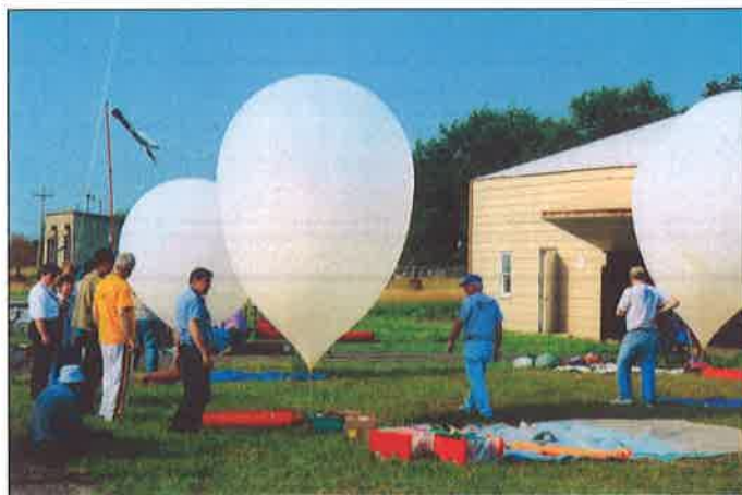
Some launches, just after the balloons have been filled. Until they are tied and taped shut, the balloons are secured to 120 lb. helium bottles to anchor them while the rest of the NS craft is being prepped.
