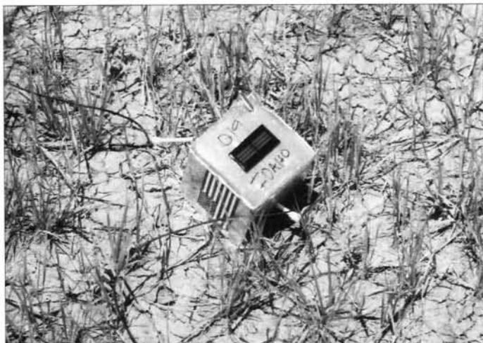
A BalloonSat after recovery. BalloonSats do not carry independent trackers, but rely on the NS craft they are attached to. BalloonSats are designed and built by university students as part of the Space Grant Consortium.
