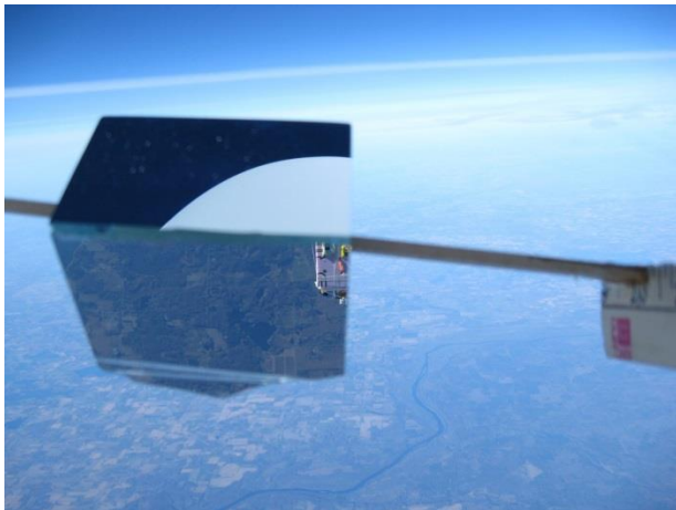
Fig. 6 (2008) Up/out/down simultaneous views using the mirror boom from 37,000 ft.
