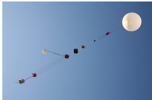
Fig. 12 (2010) Payload stack in flight, just after release into a cloudless sky. One payload made use of a horizontal boom with a small balloon attached – another IGL experiment
