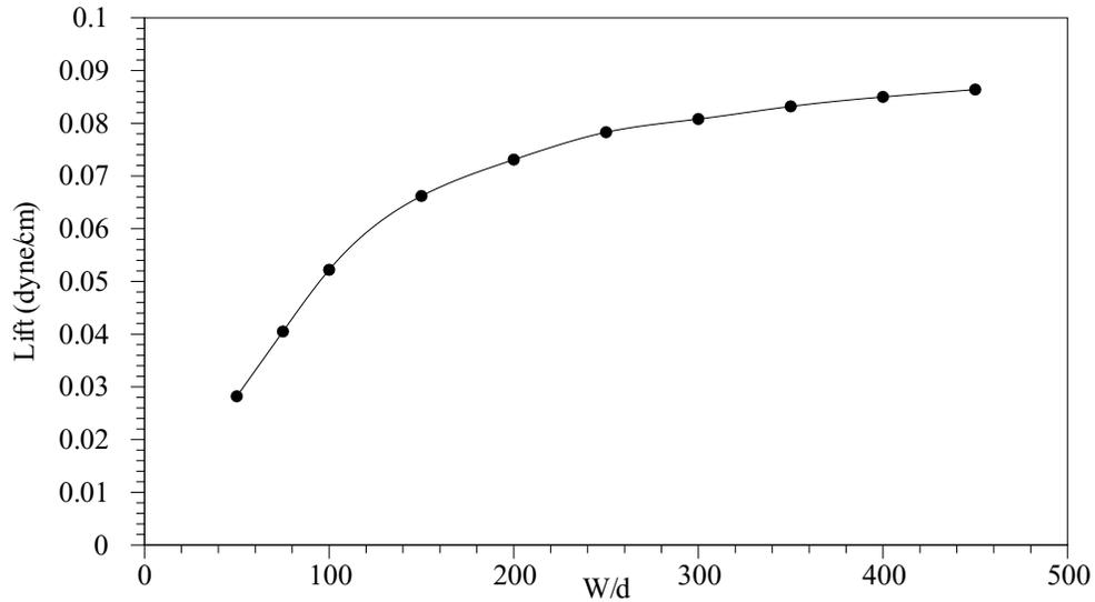
Figure 7. Lift vs. domain size for a particle in an unbounded linear shear flow.
