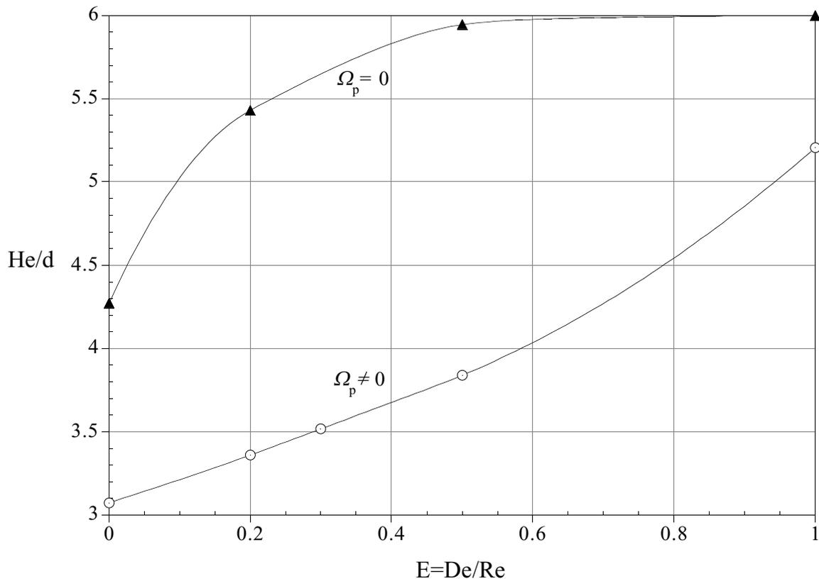
Figure 25. Lift-off of a circular particle from a horizontal wall in a Poiseuille flow of an Oldroyd-B fluid ( $W/d = 12$ ,  $l/d = 22$ ,  $\eta = 1.0$  poise,  $d = 1.0$  cm,  $R = 0.60$ ).
