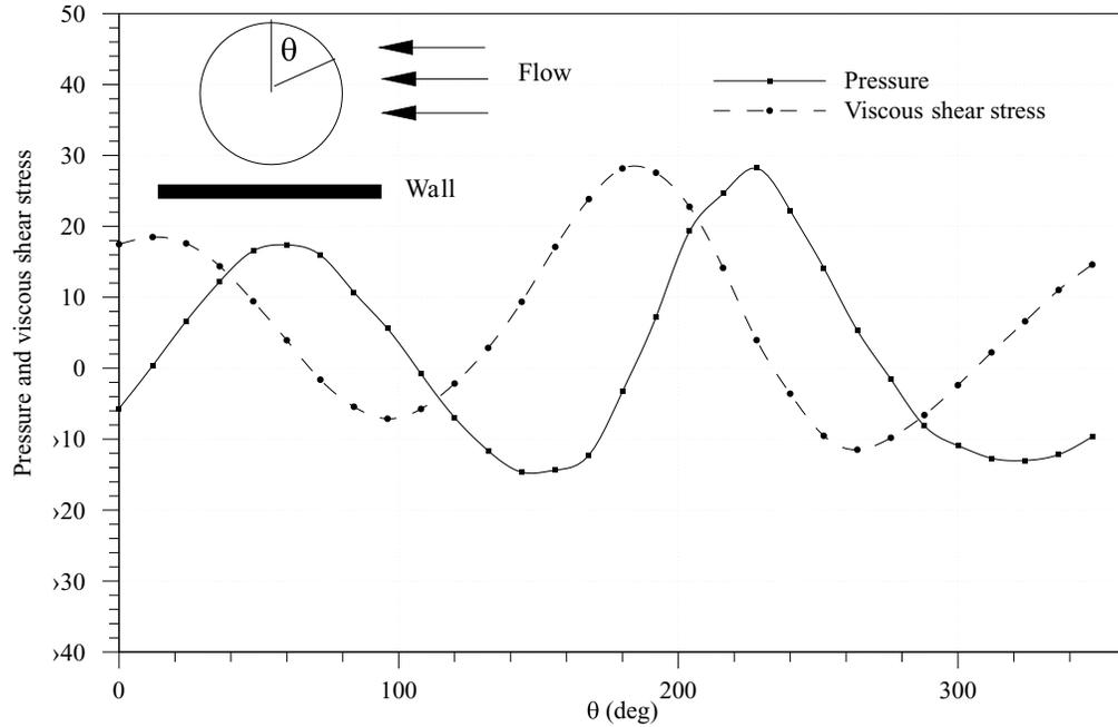
Figure 20(e). Distributions of pressure and viscous shear stress on the surface of a non-rotating circular particle in a Poiseuille flow of a Newtonian fluid.  $W/d = 12$ ,  $l/d = 22$ ,  $d = 1.0$  cm,  $\rho_p/\rho_f = 1.01$ ,  $R = 27$  (after bifurcation).
