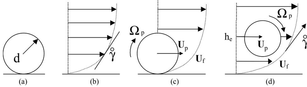
Figure 3. Lift-off and levitation to equilibrium.
