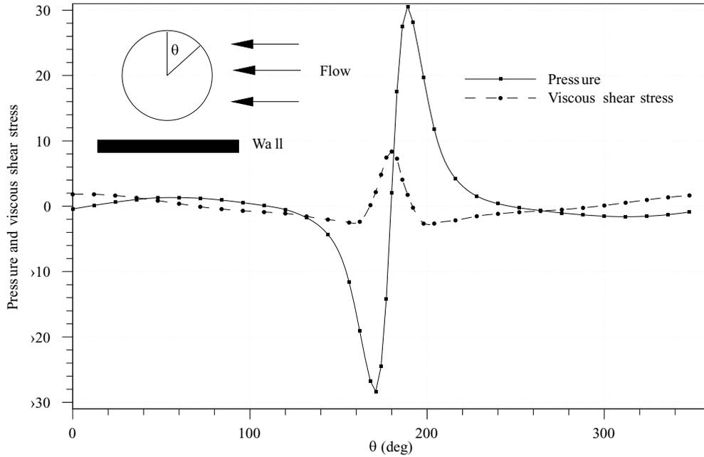
Figure 30(a). Distributions of pressure and viscous shear stress on the surface of a freely rotating circular particle in a Poiseuille flow of a Newtonian fluid.  $W/d = 12$ ,  $l/d = 22$ ,  $d = 1.0$  cm,  $\rho_p/\rho_f = 1.001$ ,  $R = 0.6$ . The particle does not lift off.
