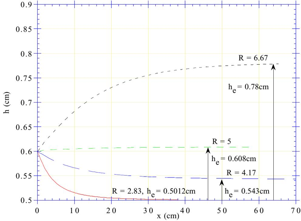
Figure 9. Cross stream migration of a single particle ( $\rho_p > \rho_f$ ). A single particle of diameter  $d = 1$  cm is released at a height of  $0.6d$  in a Poiseuille flow. It migrates to an equilibrium height  $h_e$ .
