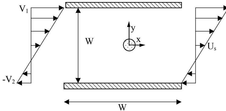
Figure 6. Computational domain for the simulation of linear shear flows around a circular particle.
