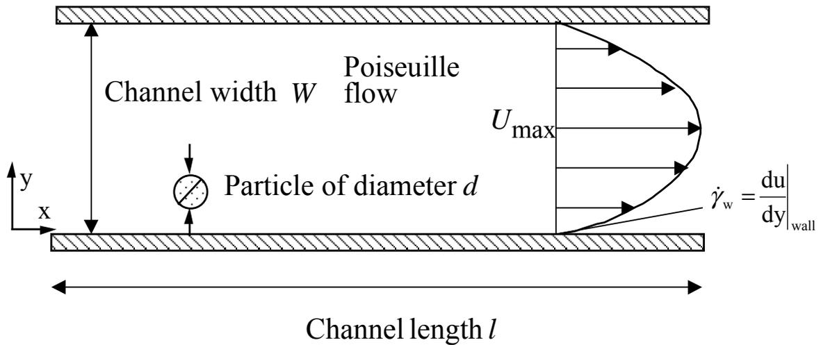
Figure 1. Computational domain for the lift-off of a single particle in plane Poiseuille flow.
