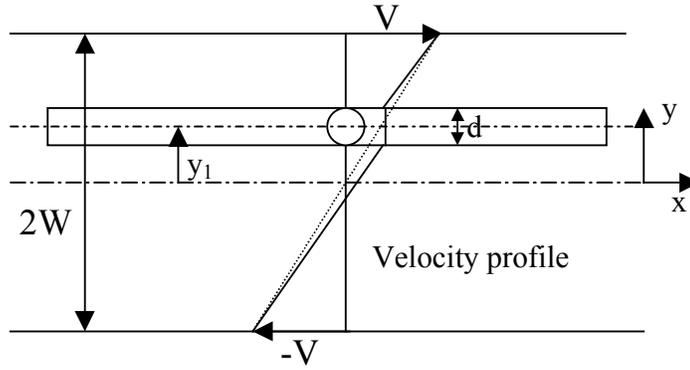
Figure 8. A long rectangular particle in a steady Couette flow. The dotted line represents the undisturbed velocity profile whereas the solid line represents the velocity profile in the presence of the long particle.
