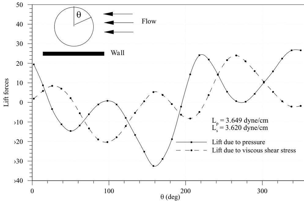
Figure 20(d). The distribution of lift forces on the surface of a freely rotating circular particle in a Poiseuille flow of a Newtonian fluid.  $W/d = 12$ ,  $l/d = 22$ ,  $d = 1.0$  cm,  $\rho_p/\rho_f = 1.01$ ,  $R = 27$  (after bifurcation).
