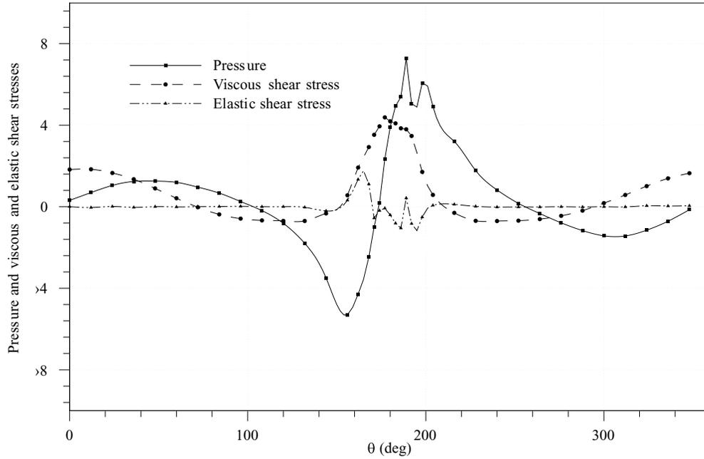
Figure 30(e). Distributions of pressure and viscous and elastic shear stresses on the surface of a lifted circular particle in a Poiseuille flow of an Oldroyd-B fluid.  $W/d = 12$ ,  $l/d = 22$ ,  $d = 1.0$  cm,  $\rho_p/\rho_f = 1.001$ ,  $R = 0.6$ ,  $E = 0.5$ ,  $\Omega_p = 0$ .
