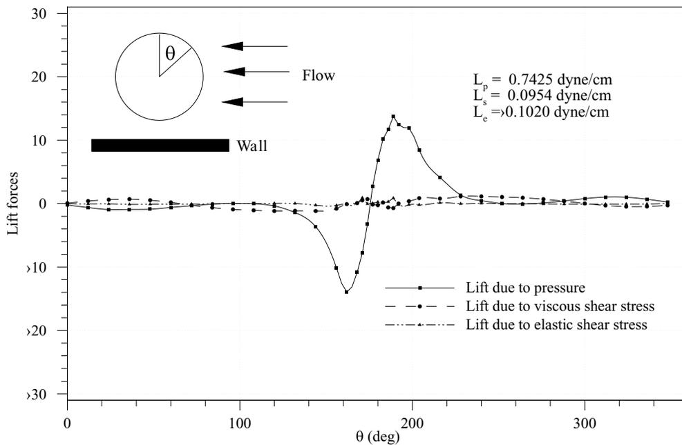
Figure 30(d). The distribution of lift forces on the surface of a freely rotating particle.  $W/d = 12$ ,  $l/d = 22$ ,  $d = 1.0$  cm,  $\rho_p/\rho_f = 1.001$ ,  $R = 0.6$ ,  $E = 0.5$ . The particle lifts off.
