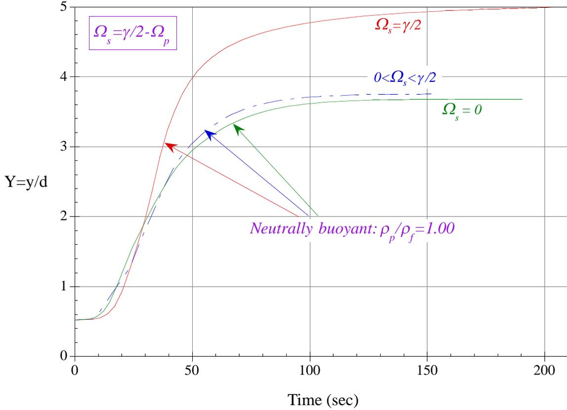
Figure 17. Rise vs. time for a neutrally buoyant particle ( $R = 5.4$ ,  $W/d = 12$ ,  $l/d = 22$ ,  $\eta = 1$  poise,  $d = 1$  cm).
