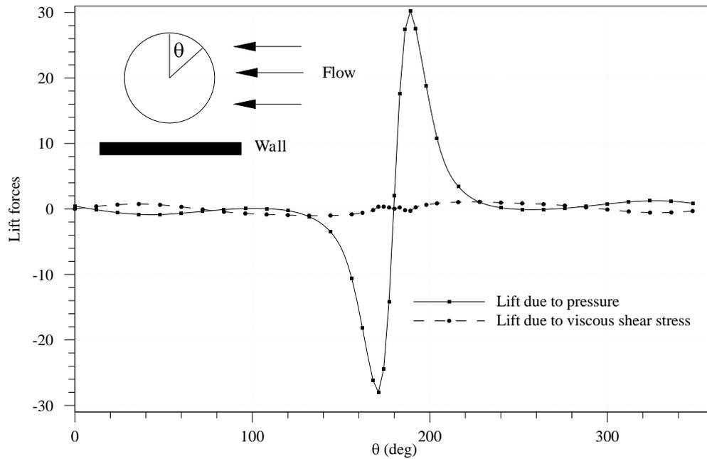
Figure 30(c). The distribution of lift forces on the surface of a freely rotating particle.  $W/d = 12$ ,  $l/d = 22$ ,  $d = 1.0$  cm,  $\rho_p/\rho_f = 1.001$ ,  $R = 0.6$ , Newtonian fluid. The particle does not lift off.
