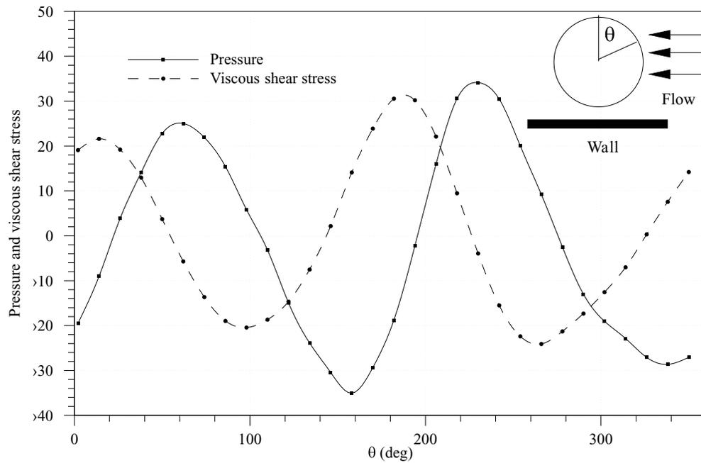
Figure 20(b). Distributions of pressure and viscous shear stress on the surface of a freely rotating circular particle in a Poiseuille flow of a Newtonian fluid.  $W/d = 12$ ,  $l/d = 22$ ,  $d = 1.0$  cm,  $\rho_p/\rho_f = 1.01$ ,  $R = 27$  (after bifurcation).
