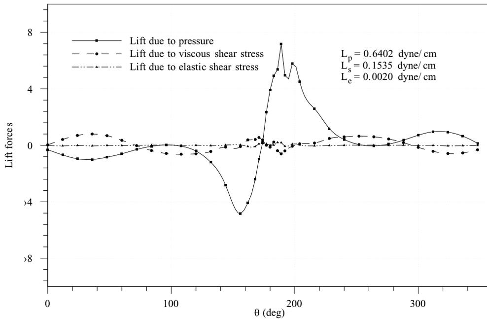
Figure 30(f). The distribution of lift forces on the surface of a lifted circular particle in an Oldroyd-B fluid.  $W/d = 12$ ,  $l/d = 22$ ,  $d = 1.0$  cm,  $\rho_p/\rho_f = 1.001$ ,  $R = 0.6$ ,  $E = 0.5$ ,  $\Omega_p = 0$ .
