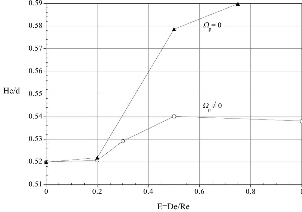
Figure 28. Lift-ff of a circular particle from a horizontal wall in a Poiseuille flow of an Oldroyd-B fluid ( $W/d = 12$ ,  $l/d = 22$ ,  $\eta = 1.0$  poise,  $d = 1.0$  cm,  $\rho_p = 1.001$  g/cc).
