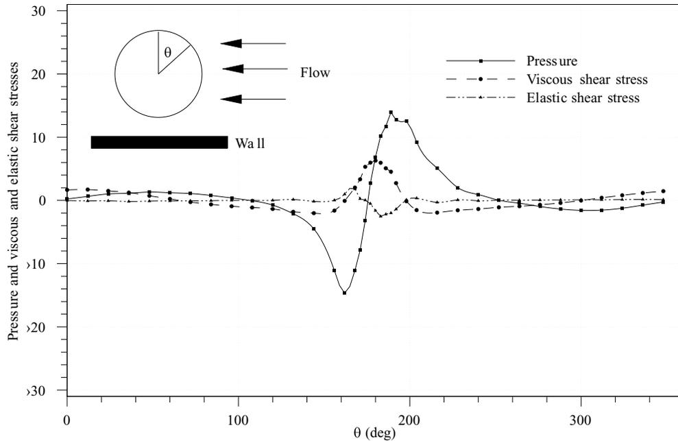
Figure 30(b). Distributions of pressure and viscous and elastic shear stresses on the surface of a freely rotating circular particle in a Poiseuille flow of an Oldroyd-B fluid.  $W/d = 12$ ,  $l/d = 22$ ,  $d = 1.0$  cm,  $\rho_p/\rho_f = 1.001$ ,  $R = 0.6$ ,  $E = 0.5$ . The particle lifts off.
