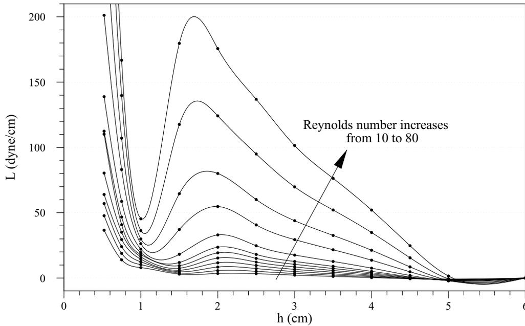
Figure 22. The hydrodynamic lift force on the particle as a function of the height of its center from the bottom wall at different shear Reynolds numbers. The bottom wall is  $h = 0$  cm and the channel centerline is  $h = 6$  cm.
