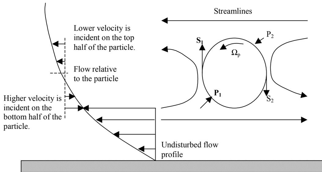
Figure 21. Cartoon depicting the fluid velocity and the streamlines relative to a particle in a plane Poiseuille flow. The fluid approaches the particle with higher velocity in the bottom half of the particle. Consequently, the pressure  $P_1$  (in bold) is greater than  $P_2$  and the viscous shear stress  $S_1$  (in bold) is greater than  $S_2$ .
