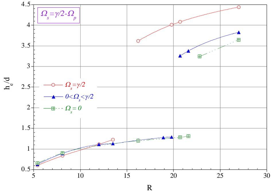
Figure 14. Lift-off of a circular particle from a horizontal wall in a Poiseuille flow of a Newtonian fluid ( $W/d = 12$ ,  $l/d = 22$ ,  $\eta = 1.0$  poise,  $d = 1$  cm,  $\rho_p = 1.01$  g/cc).
