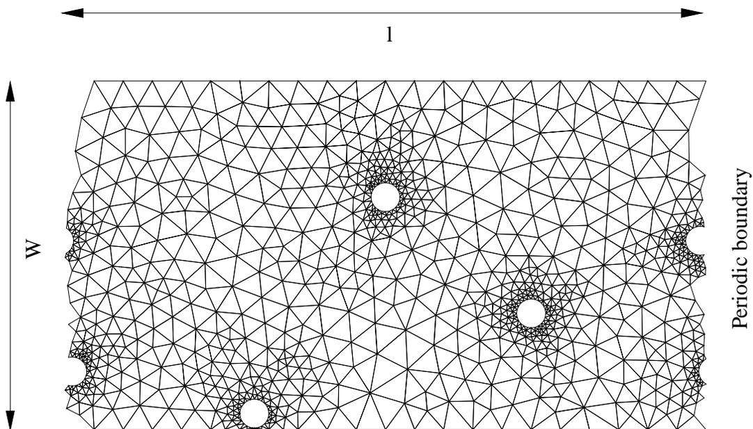
*Figure 2. Unstructured mesh in a periodic domain with many particles. In our simulations there is one particle in the domain.*
