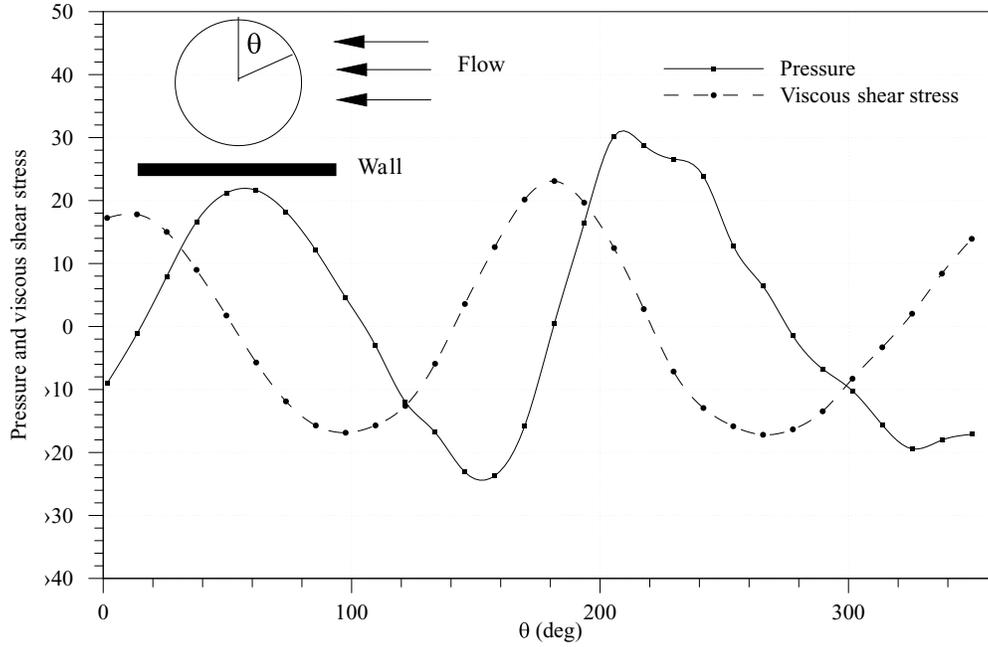
Figure 20(a). Distributions of pressure and viscous shear stress on the surface of a freely rotating circular particle in a Poiseuille flow of a Newtonian fluid.  $W/d = 12$ ,  $l/d = 22$ ,  $d = 1.0$  cm,  $\rho_p/\rho_f = 1.01$ ,  $R = 8.1$  (before bifurcation).
