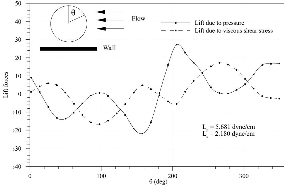
Figure 20(c). The distribution of lift forces on the surface of a freely rotating circular particle in a Poiseuille flow of a Newtonian fluid.  $W/d = 12$ ,  $l/d = 22$ ,  $d = 1.0$  cm,  $\rho_p/\rho_f = 1.01$ ,  $R = 8.1$  (before bifurcation).
