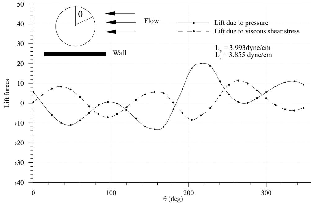
Figure 20(f). The distribution of lift forces on the surface of a non-rotating circular particle in a Poiseuille flow of a Newtonian fluid.  $W/d = 12$ ,  $l/d = 22$ ,  $d = 1.0$  cm,  $\rho_p/\rho_f = 1.01$ ,  $R = 27$  (after bifurcation).
