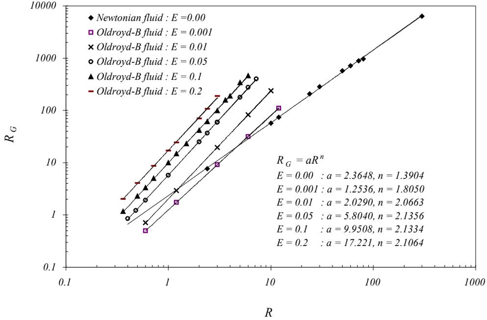
Figure 1 (b). The plot of  $R_G$  vs. the shear Reynolds number  $R$  for lift-off on a logarithmic scale for a Newtonian and an Oldroyd-B fluid at different values of  $\lambda_2/\lambda_1$ .
