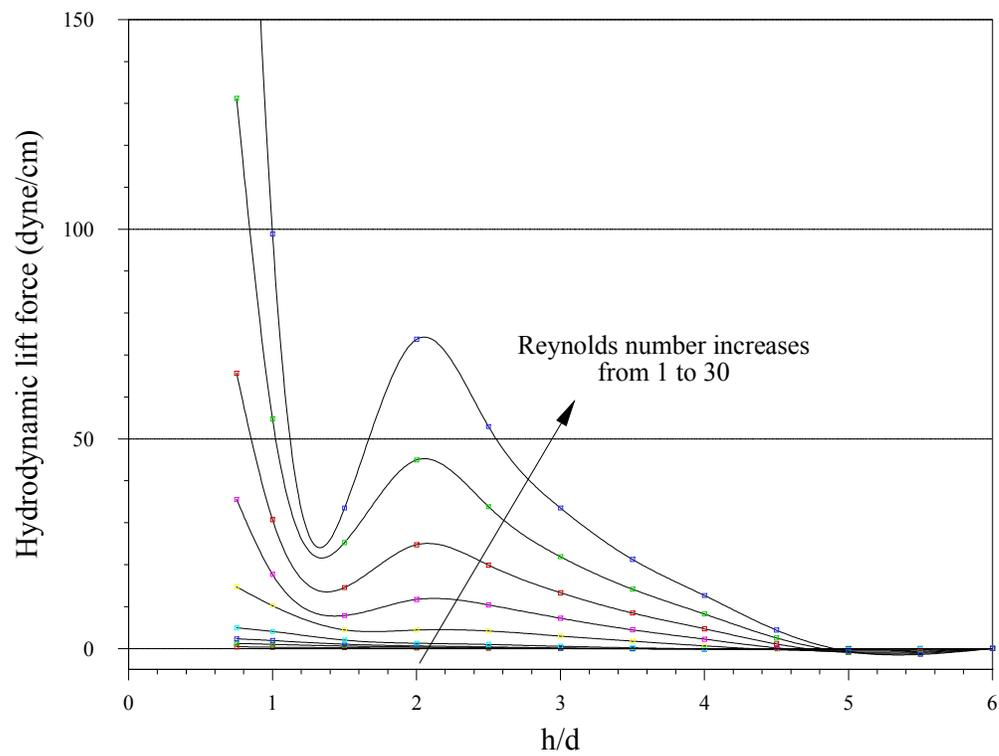
Figure 6. Finding the equilibrium height of a particle of a given density at different values of shear Reynolds number.
