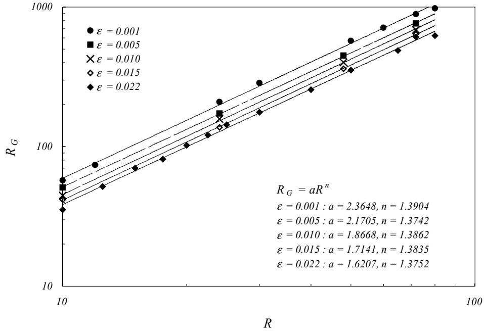
Figure 3 (b). The plot of  $R_G$  vs. the critical shear Reynolds number  $R$  for lift-off on a logarithmic scale at Oldroyd-B fluid for various gap sizes.
