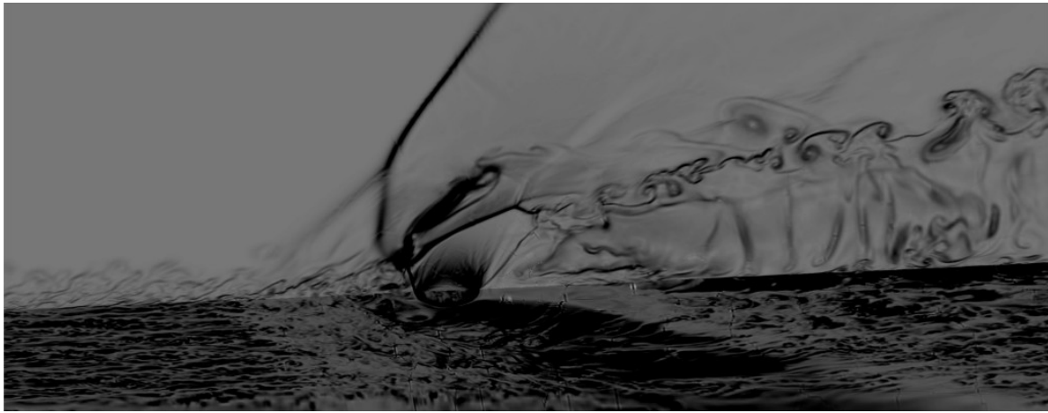
Figure 6. 3D view of instantaneous density gradient magnitude contours.
