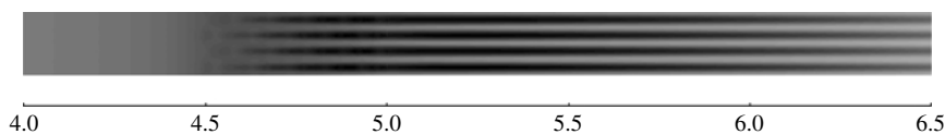
FIGURE 25. Instantaneous contours of streamwise velocity from simulation 4 in table 2 show that flow remains laminar past the roughness region. Mach number is 2.9, Re = 635\,000/\text{inch} , and the roughness amplitude k = 0.005 .
