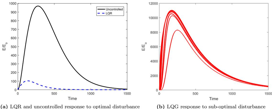
**Figure 1:** Spanwise wave case  $\alpha = 0, \beta = 1$  at  $Re = 3000$ . Under critical Reynolds number, the open-loop system is linearly stable with high TEG (solid). A selected LQR controller can reduce the amount of the maximum TEG to around 103.5 (dashed). But LQG result in high levels of TEG.
