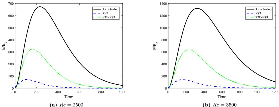
**Figure 3:** LQR and SOF-LQR both exhibit robust TEG reduction with Reynolds number variations.
