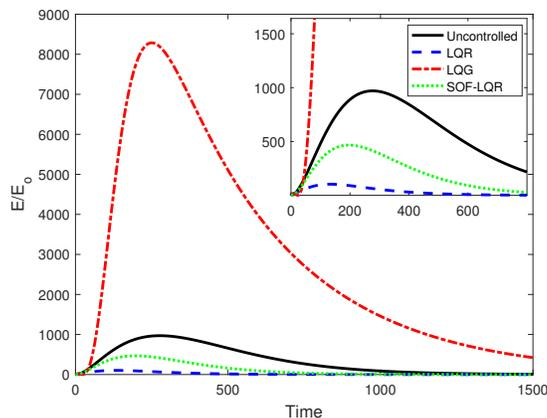
**Figure 2:** Spanwise wave case  $\alpha = 0$ ,  $\beta = 1$  at  $Re = 3000$ . Though cannot work as well as LQR, SOF-LQR still performances better than LQG controllers regarding to TEG suppression.
