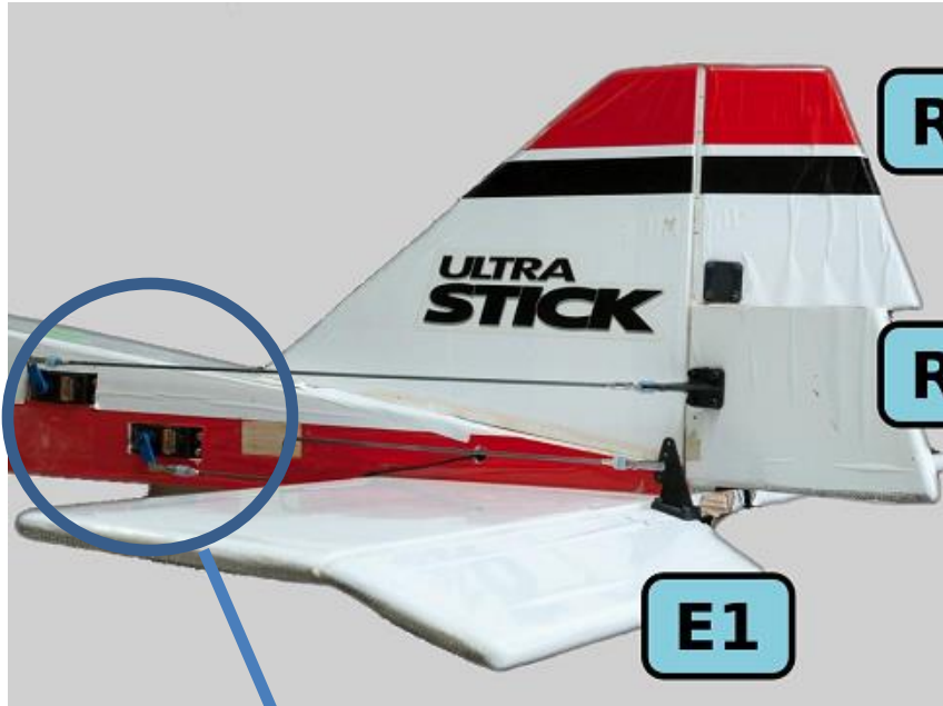
Low-cost servos drive the surfaces
