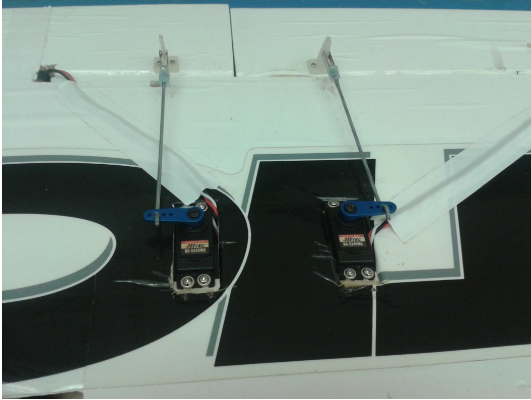
Figure 15: A pair of wing servos, one used to control the left aileron, and the other used to actuate the left flap.
