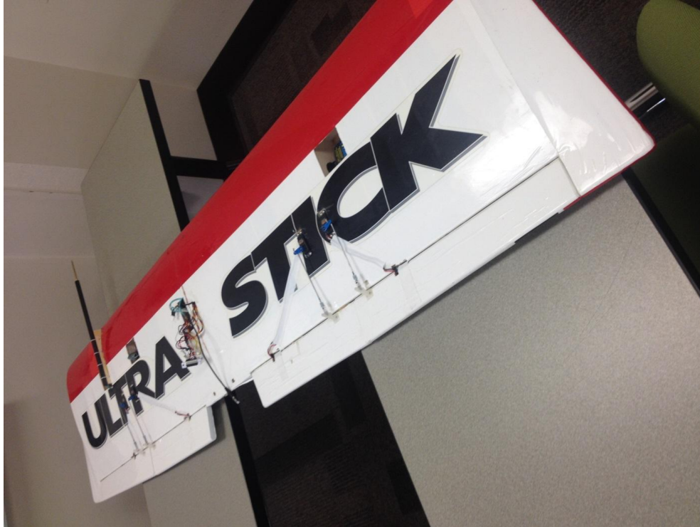
Figure 18: The full wing once completed. The pitot tube mount and the slot for the GPS antenna can be seen, as well as the center hole for all of the wiring meant to connect to the flight computer. The servos and potentiometers attaching to the control surfaces are also visible.
