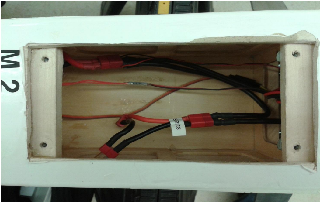
Figure 6: The front hatch cutout in the nose of the aircraft, allowing access to the motor batteries and connecting wires. The wooden mounts and screw holes where the hatches are fastened can be seen on either side of the cutout.
