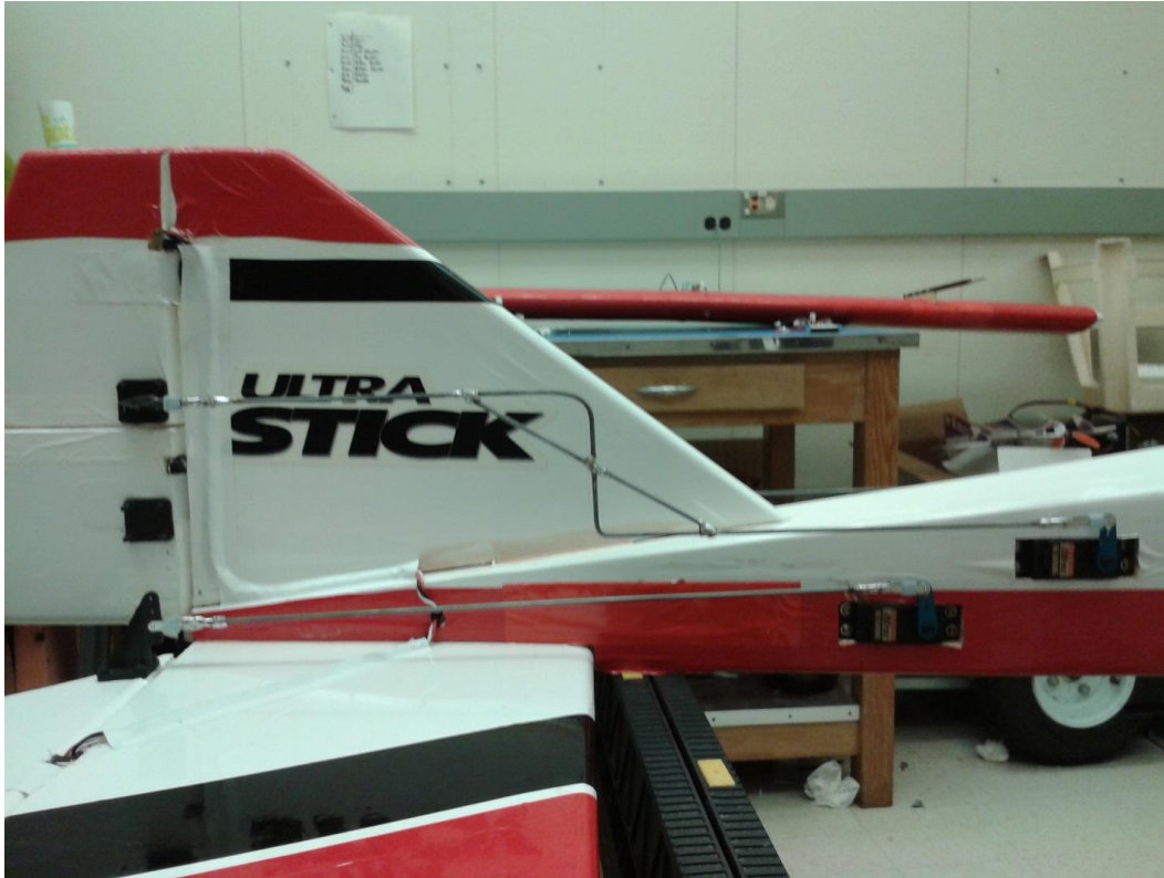
Figure 11: The two starboard control rods used to actuate the right elevator and top rudder. The top control rod is bent to accommodate the height difference between the top rudder control horn and its servo motor arm. The reinforcing diagonal cross piece is also shown.
