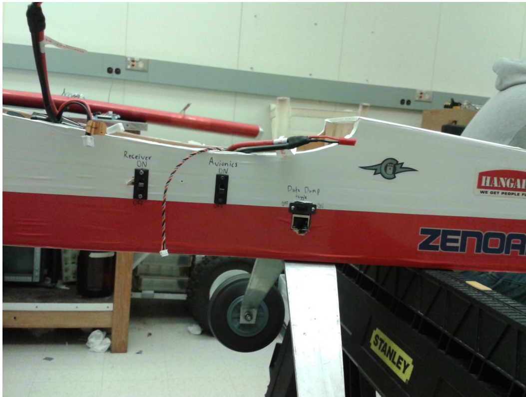
Figure 13: The receiver, avionics, and data dump switches mounted on the outside wall of the aircraft, along with the landing gear bracket.
