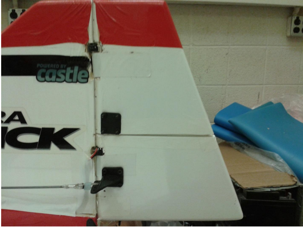
Figure 8: A picture of the horizontal cut made to separate the rudder into two separate control surfaces.
