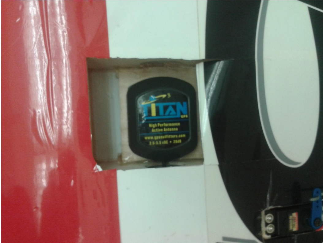
Figure 16: A picture illustrating the wooden mount and placement of the GPS antenna within the wing.
