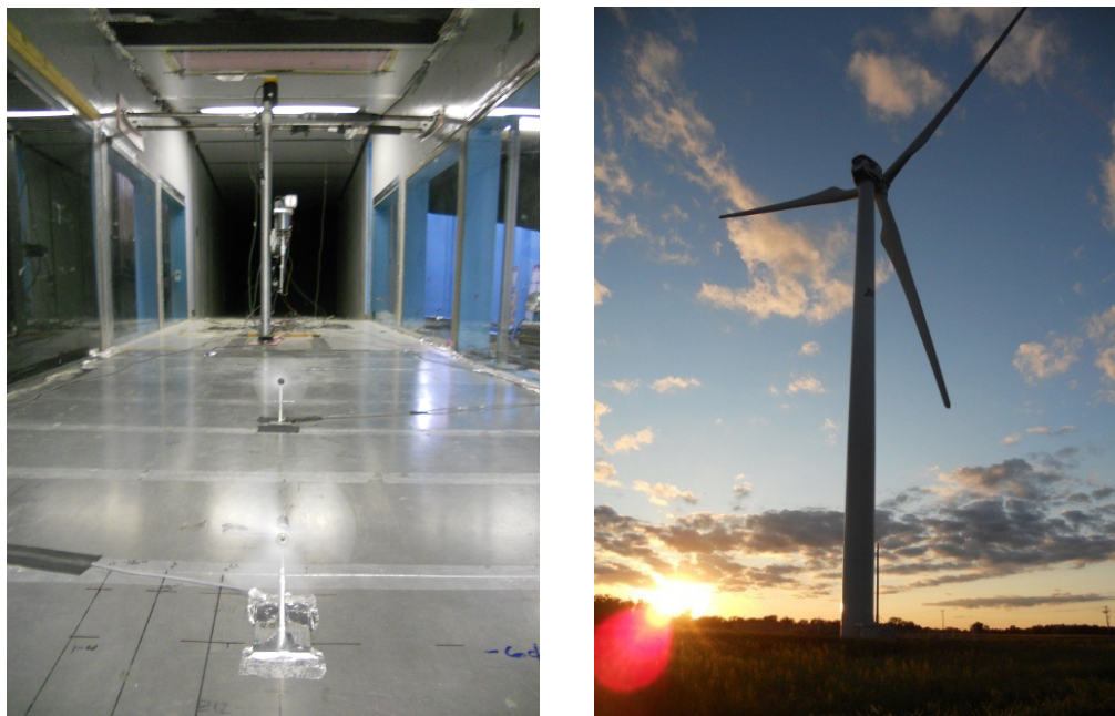
Figure 4. Two turbine setup in the SAFL wind tunnel (left) and the 2.5 MW Clipper turbine at UMore Park (right)
