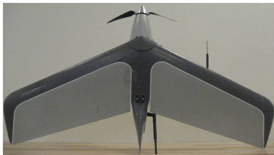
(a) The aircraft has two elevons and a motor.
