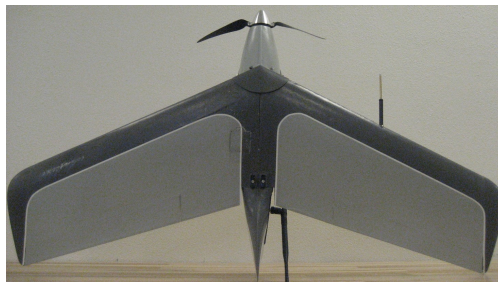
Fig. 1 The Sentera Vireo – the small, rudderless, fixed-wing UAS considered in this paper.
