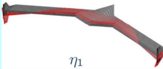
Symmetric 1 st Bending ~6Hz
