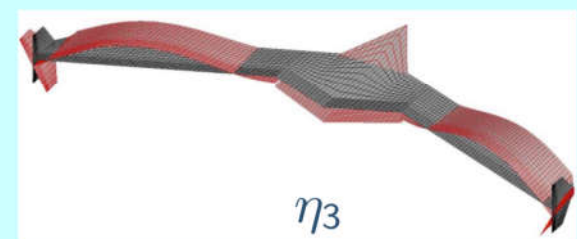
Symmetric 2 nd Bending ~19.5Hz
