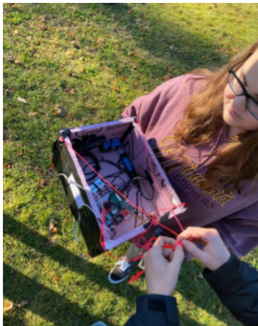
The payload on flight day with all interior items secured (except batteries). Paracord strapping is being untangled in order to secure our payload to Team B's payload.
