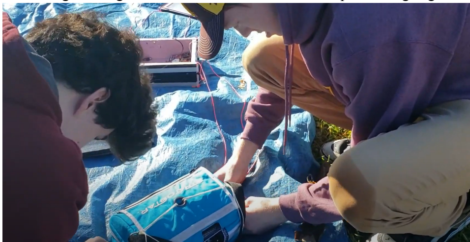
Tying 550 cords to the keyrings in order to assemble all of the payloads in the stack.
