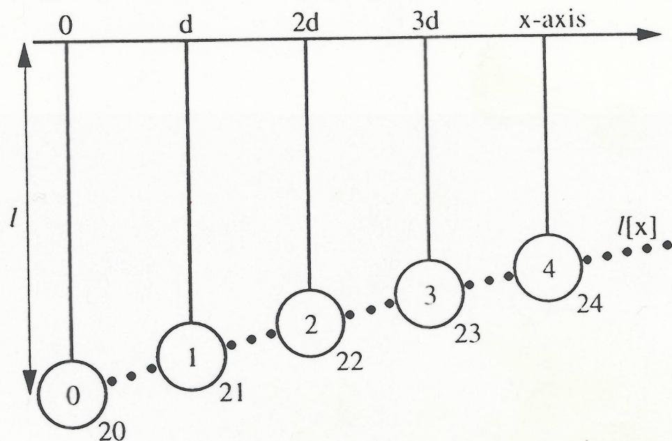
Tune pendula so that in time  $\Gamma$  (about 20 s for our apparatus) the longest pendulum goes through  $N$  cycles ( $N=20$ ), the next goes through  $N+1$ , the next  $N+2$ , etc.
