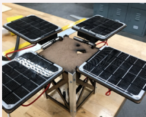
Assembly of HDF and aluminum payload with 6V solar panels secured and deployed.
