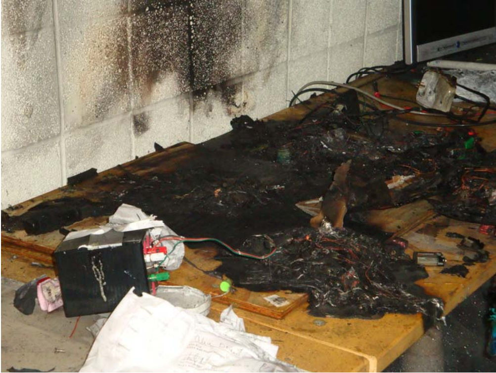
Fire damage 398 Shepherd Labs – source on table
