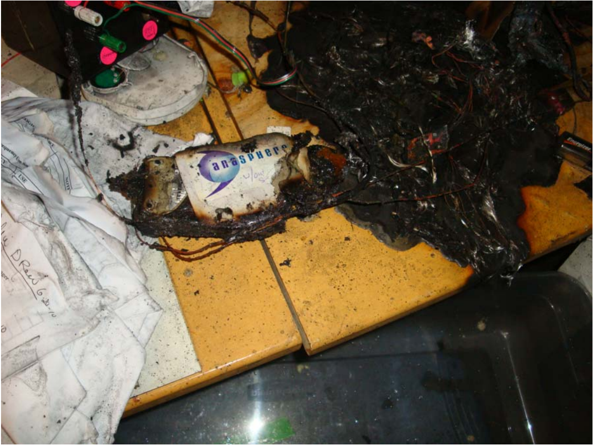
Possible source – Battery charger moved from middle of burnt material
