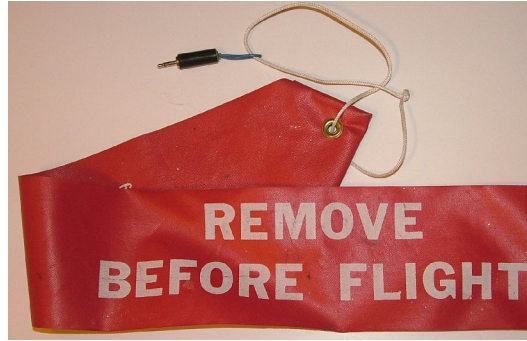
Figure 34. A brightly colored orange ribbon tied to the Commit Pin. This ribbon ensures that no one forgets to pull the Commit Pin at launch.
