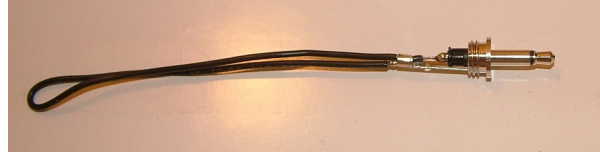
Figure 24. The phono plug after soldering its shorting wire.
