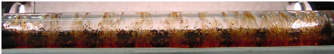
Figure 26. Segregation of two types of particles in water. The filling level is 0.357. The black is a silicon particle with \rho_p = 3.07 \text{ g/cm}^3 , average diameter d_p = 0.05 \text{ cm} , and its concentration is 4%. The brown is a resin particle with \rho_p = 1.13 \text{ g/cm}^3 , average diameter d_p = 0.065 \text{ cm} , and its concentration is 16%. The rotational speed is 306 rpm.
