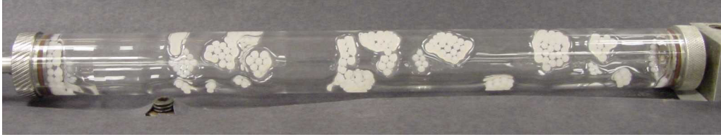
Figure 15. Clustering of particles due to capillarity. The fluid is glycerin with a density of 1.173 \text{ g/cm}^3 , a viscosity of 1490 \text{ cp} , and a surface tension of 41.46 \text{ mN/m} . The particles are white Nylon particles with a density of 1.170 \text{ g/cm}^3 and a diameter of 0.314 \text{ cm} . The filling level of the fluid is 8.2\% and the particle concentration is 54.2\% . The rotating speed \Omega=5.45 \text{ rpm} , \beta=1.127 , average film thickness D_a=0.585 \text{ mm} , minimum film thickness D_{\min}=0.526 \text{ mm} , D_{\min}/d_p=0.176 . Clusters of particles form about 5 minutes after starting of rotation. Bands form occasionally but are not stable.
