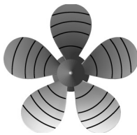
FIG. 2. A schematic showing how the propeller is broken down into strips for the case of five strips per blade resulting in 25 strips in total. The strips are equal in thickness along the radial direction.
