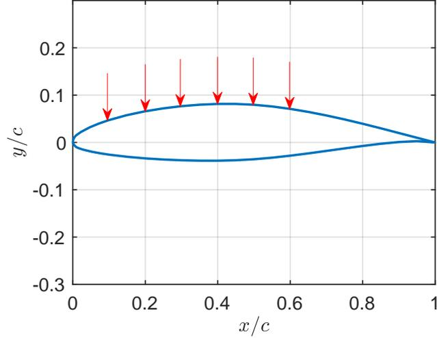
Figure 1: NACA 65(1)-412 airfoil. The positions  $x/c = \{.1, .2, .3, .4, .5, .6\}$ , on the upper surface of the airfoil correspond to the various actuator locations. These are indicated by the red arrows.
