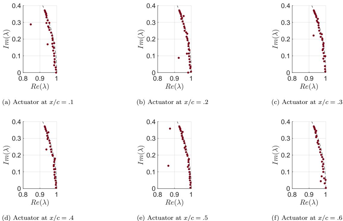
Figure 4: System poles of (discrete-time) minimal realization computed from lift pulse response data for each actuator location using ERA. Some poles are outside the unit circle for all locations.
