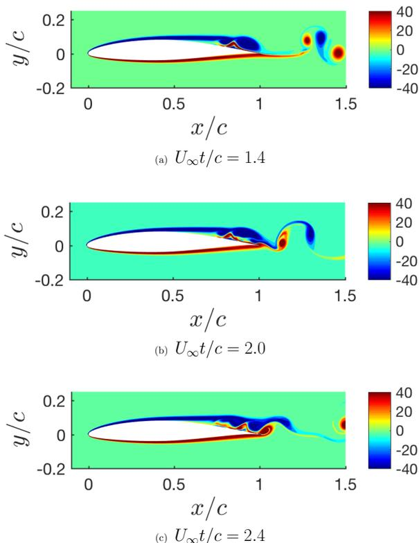
Figure 3: NACA 65(1)-412,  $\alpha = 4^\circ$ ,  $Re_c = 20,000$ , Vorticity field at (a)  $U_\infty t/c = 1.4$ , (b)  $U_\infty t/c = 2.0$  and (c)  $U_\infty t/c = 2.4$  for the case with a pulse actuation at  $x/c = 0.4$ .
