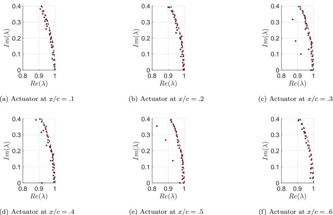
Figure 7: System poles of (discrete-time) minimal realization computed from separation angle pulse response data for each actuator location using ERA. Some poles are outside the unit circle for all locations.
