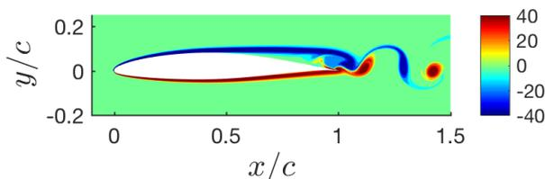
Figure 2: NACA 65(1)-412,  $\alpha = 4^\circ$ ,  $Re_c = 20,000$ , Vorticity field at  $U_\infty t/c = 0.60$  for the baseline case.
