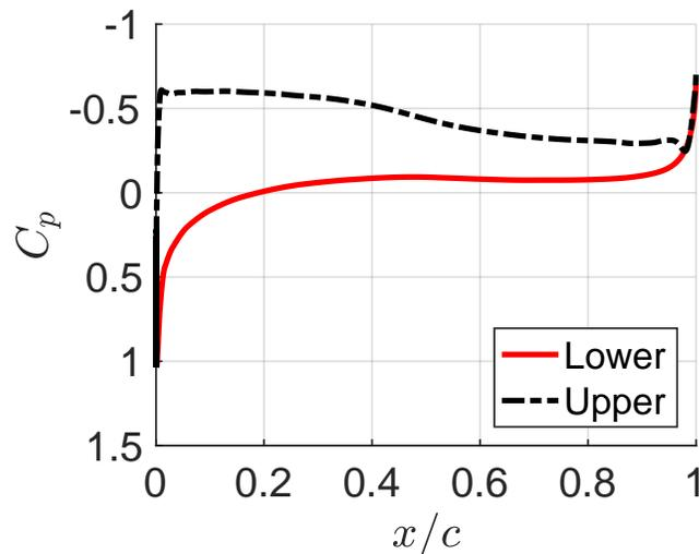
Figure 10: Pressure coefficients for the upper and lower surface of the airfoil for the baseline flow just before pulse actuation is applied. This corroborates the findings of the optimality study as the optimal locations are, indeed, more sensitive to the initial instability in the laminar boundary layer and are able to influence the flow more directly.
