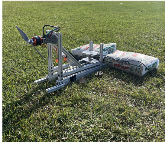
(b) Thrust stand used to perform static thrust test.
