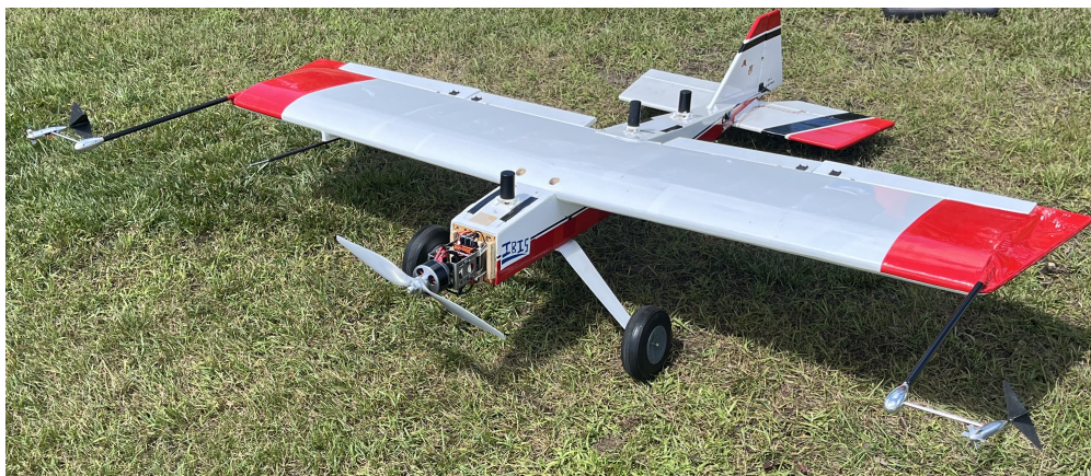
Fig. 2 Ultra Stick flight test aircraft from the University of Minnesota UAV lab. This Ultra Stick airframe, known as IBIS, is heavily instrumented as discussed in Section III.A.
