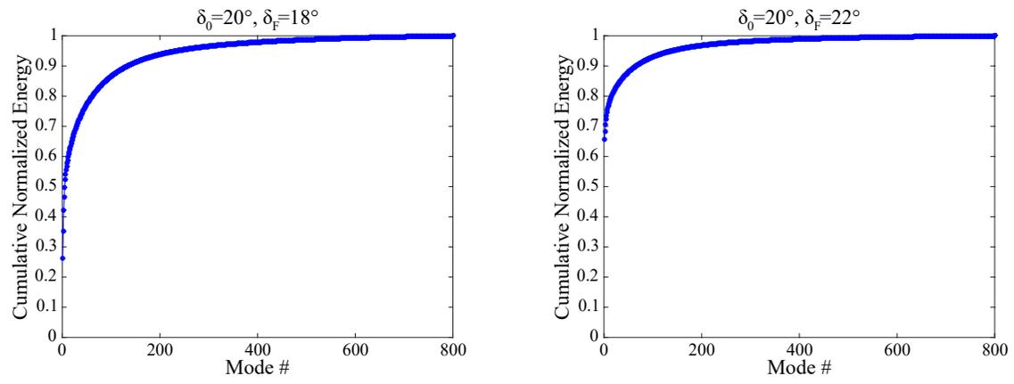
Figure 11. Cumulative normalized energy of POD modes for  $f = 6\text{Hz}$ : (left)  $\Delta\delta = -2^\circ$ , (right)  $\Delta\delta = +2^\circ$ .
