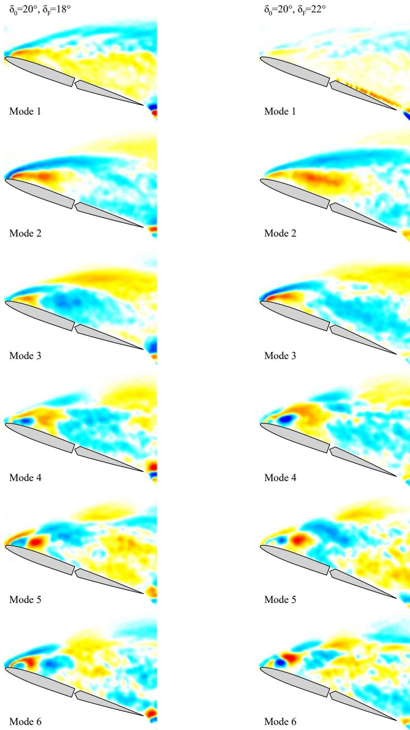
Figure 10. POD modes 1-6 for  $f = 6\text{Hz}$ : (left)  $\Delta\delta = -2^\circ$ , (right)  $\Delta\delta = +2^\circ$ .
