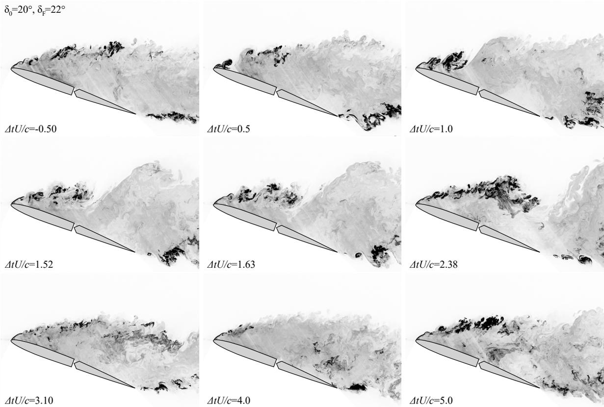
**Figure 8. Flow visualization of the temporal evolution of vortical formations in response to a single rapid flap deflection ramp:  $\Delta\delta = +2^\circ$  (net increase in positive camber) at  $f = 6\text{Hz}$ .**
