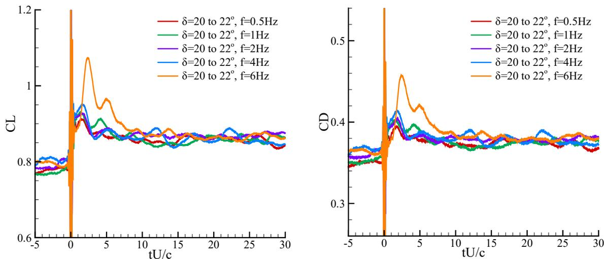
**Figure 5.** Lift and drag coefficient response to flap ramp-rate:  $\delta = [20^\circ - 22^\circ]$ ,  $f_{\text{sine}} = [0.5, 1, 2, 4, 6]$  Hz. Motion commences at  $tU/c = 0$ .
