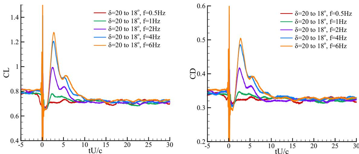
**Figure 4. Lift and drag coefficient response to flap ramp-rate:  $\delta = [20^\circ - 18^\circ]$ ,  $f_{\text{sine}} = [0.5, 1, 2, 4, 6]\text{Hz}$ . Motion commences at  $tU/c = 0$ .**
