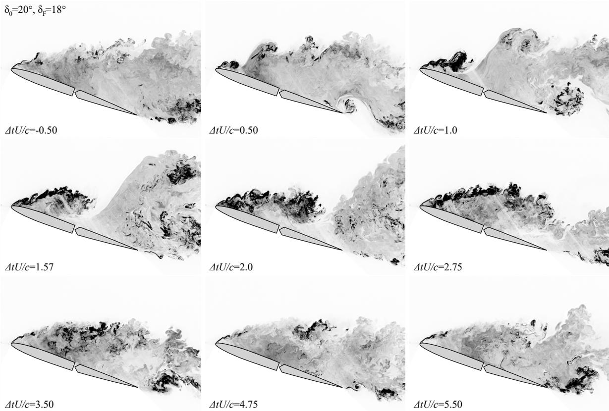
**Figure 7. Flow visualization of the temporal evolution of vortical formations in response to a single rapid flap deflection ramp:  $\Delta\delta = -2^\circ$  (net decrease in positive camber) at  $f = 6\text{Hz}$ .**
