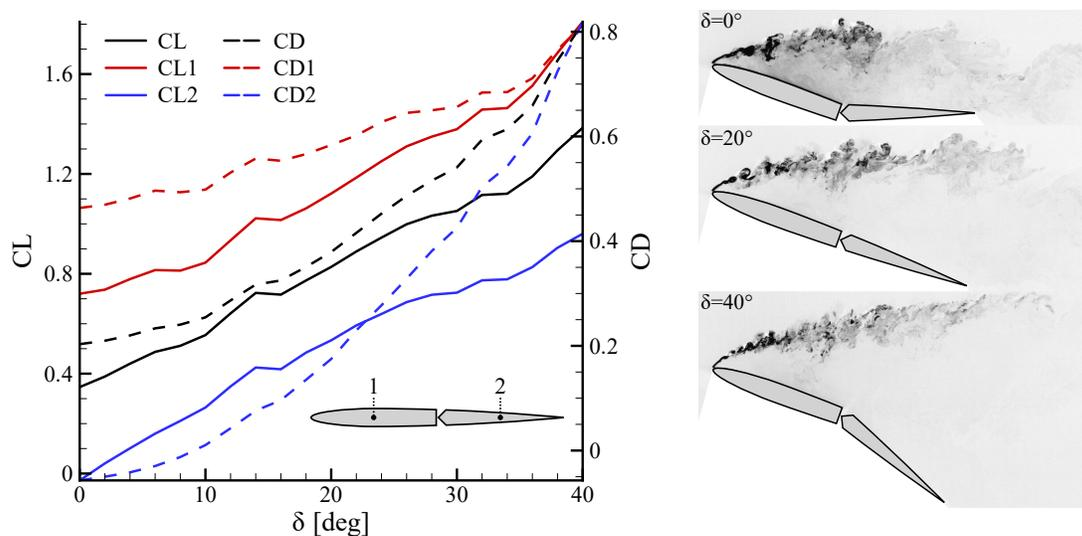
Figure 3. Static lift and drag coefficient vs deflection angle  $\delta = [0 - 40^\circ]$ : the leading element is at fixed incidence  $\alpha_{\text{LE}} = 20^\circ$ . Deflection angle  $\delta = 20^\circ$  corresponds to a planar configuration.
