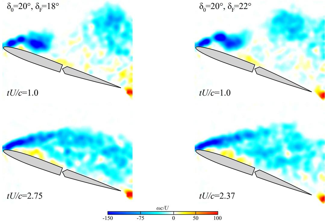
Figure 9. Vorticity fields for  $f = 6\text{Hz}$ : (left)  $\Delta\delta = -2^\circ$ , (right)  $\Delta\delta = +2^\circ$ .
