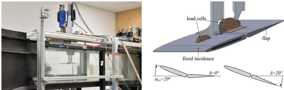
Figure 1. (left) Water tunnel facility. (right) NACA0006 configuration and angular definitions.
