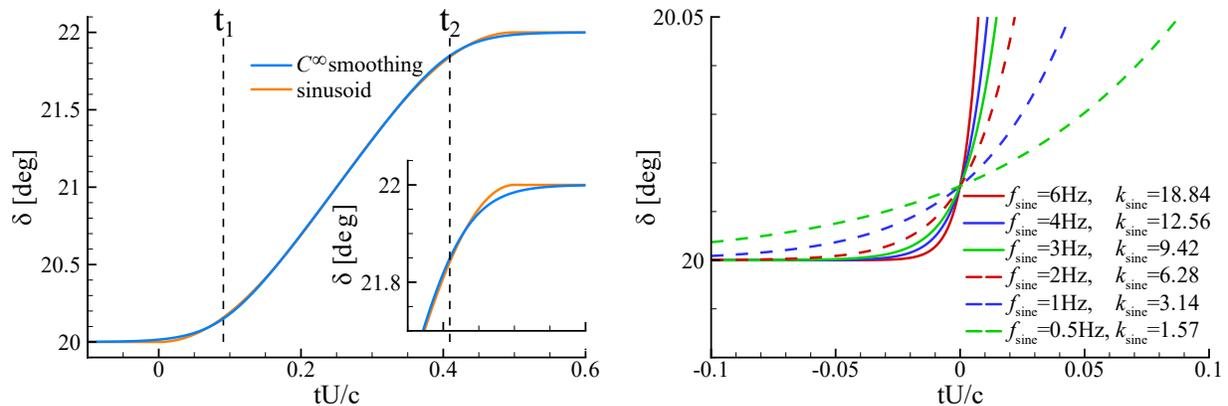
Figure 2. Typical kinematic profile for flap deflection: (*left*)  $C^\infty$ -smoothing of a sinusoidal waveform, (*right*) effects of smoothing on kinematic start time.
