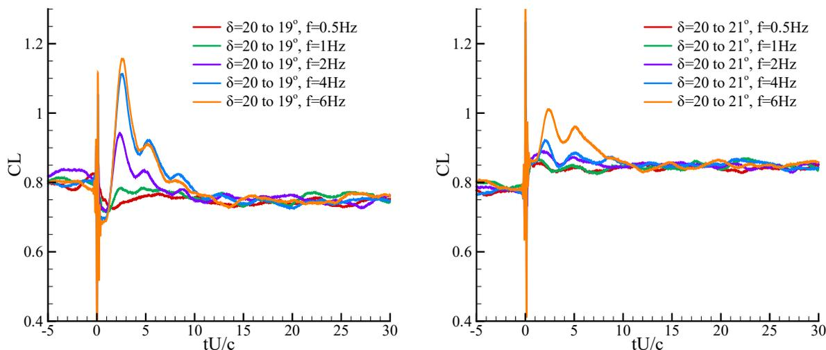
**Figure 6.** Lift coefficient response to flap ramp-rate: (left)  $\delta = [20^\circ - 19^\circ]$ , (right)  $\delta = [20^\circ - 21^\circ]$ ,  $f_{\text{sine}} = [0.5, 1, 2, 4, 6]$  Hz. Motion commences at  $tU/c = 0$ .
