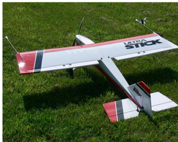
Figure 1: A picture of the UAV studied in this paper, an Ultra Stick 120. The Ultra Stick 120 is a conventional tailplane with a symmetric airfoil, marketed as a trainer-level R/C aircraft. It is relatively easy to pilot but can perform highly dynamic maneuvers that enables it to perform a wide variety of tests.
