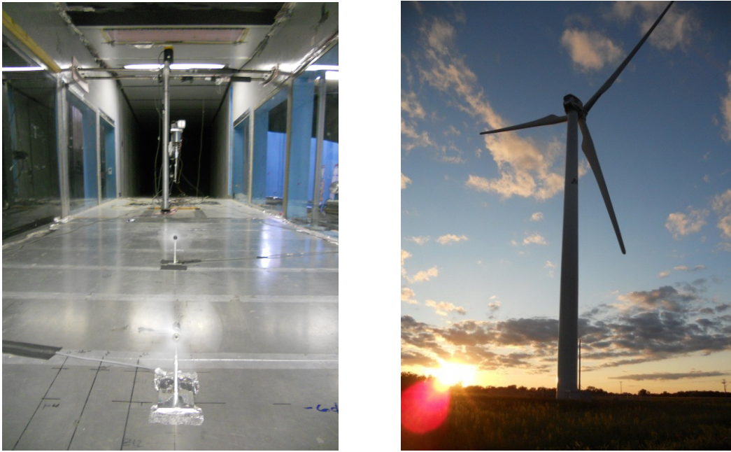
Figure 3. Two turbine setup in the SAFL wind tunnel (left) and the 2.5 MW Clipper turbine at UMore Park (right)
