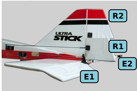
(b) Empennage with split surfaces
