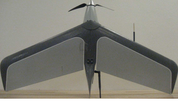
Fig. 1. The aircraft has two elevons and a motor.
