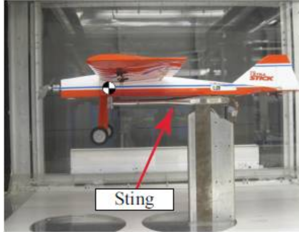
Figure 2.3: Mini Ultra Stick mounted on sting during experiments in UMN Low-Speed Wind Tunnel.
