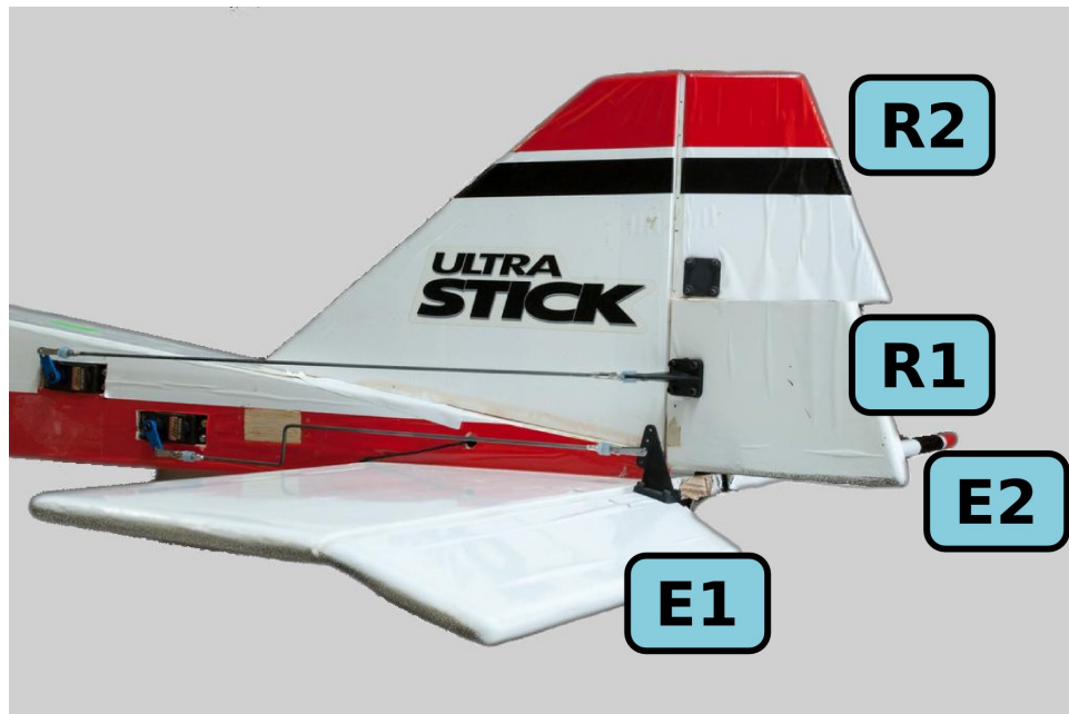
Figure 2.2: Tail of the BALDR UAV with the control surfaces labeled (E – elevator, R – rudder).
