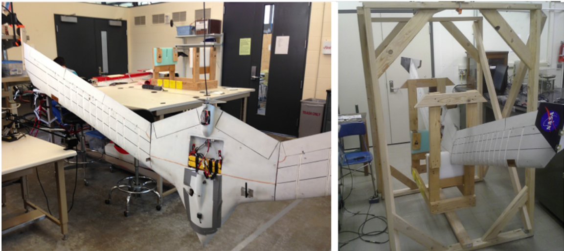
Figure 3.10: Inertia swings test setup. Source: Uninhabited aerial vehicle research laboratory at the University of Minnesota
