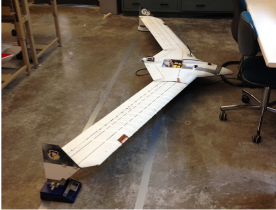
Figure 3.9: Center of gravity test setup. Source: Uninhabited aerial vehicle research laboratory at the University of Minnesota
