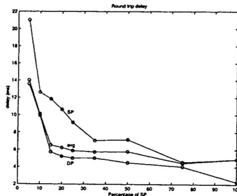
**Figure 5:** Average round-trip delay for smart (top) and dumb (bottom) packets, and average delay for all packets (center) as a function of the percentage of smart packets. These experimental results were obtained while links cpn10-cpn2, cpn2-cpn4 and cpn4-cpn5 were loaded with obstructing traffic.
