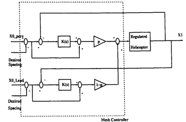
Figure 2: Mesh Controller Structure
