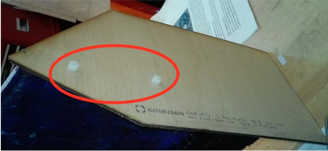
Figure 19: View of the port side winglet with the nylon bolts attaching it to the wing.
