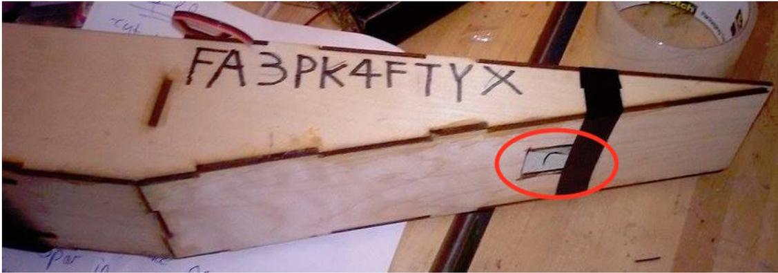
Figure 13: View of the back of the fuselage. The black tape is holding down the top plate and a hole was cut in the bottom for airflow.
