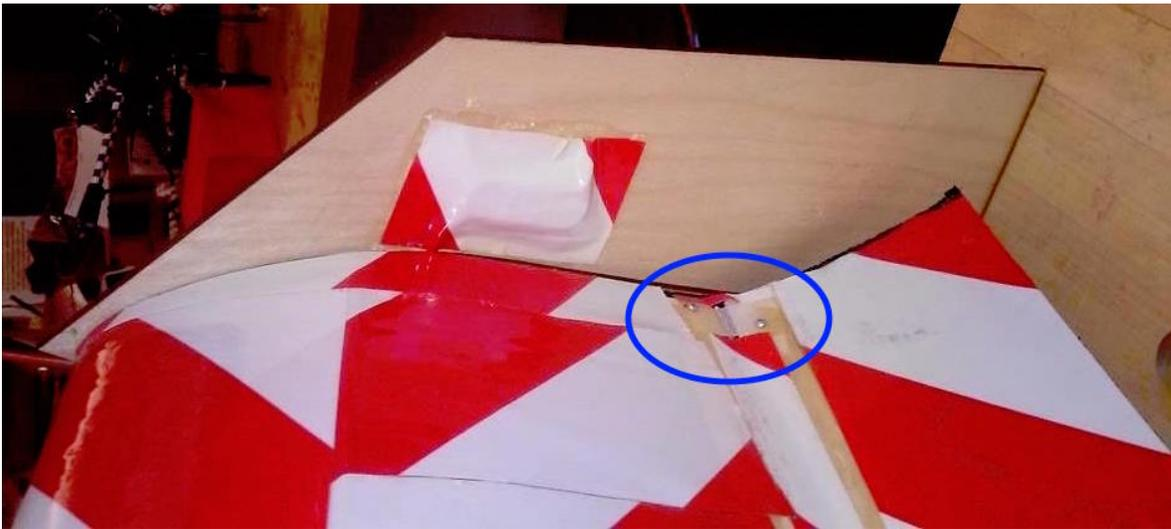
Figure 20: View of the starboard wing end and elevon. A counter weight is taped onto the winglet to balance out the pitot tube on the port side wing. In the blue circle the hinges for the elevons are shown screwed and glued into pieces of wood attached to the elevon and the wing.
