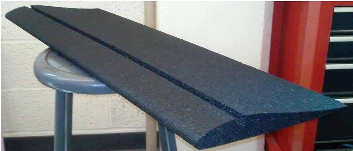
Figure 17: View of the port side foam wing with the channel cut out for the carbon spar.
