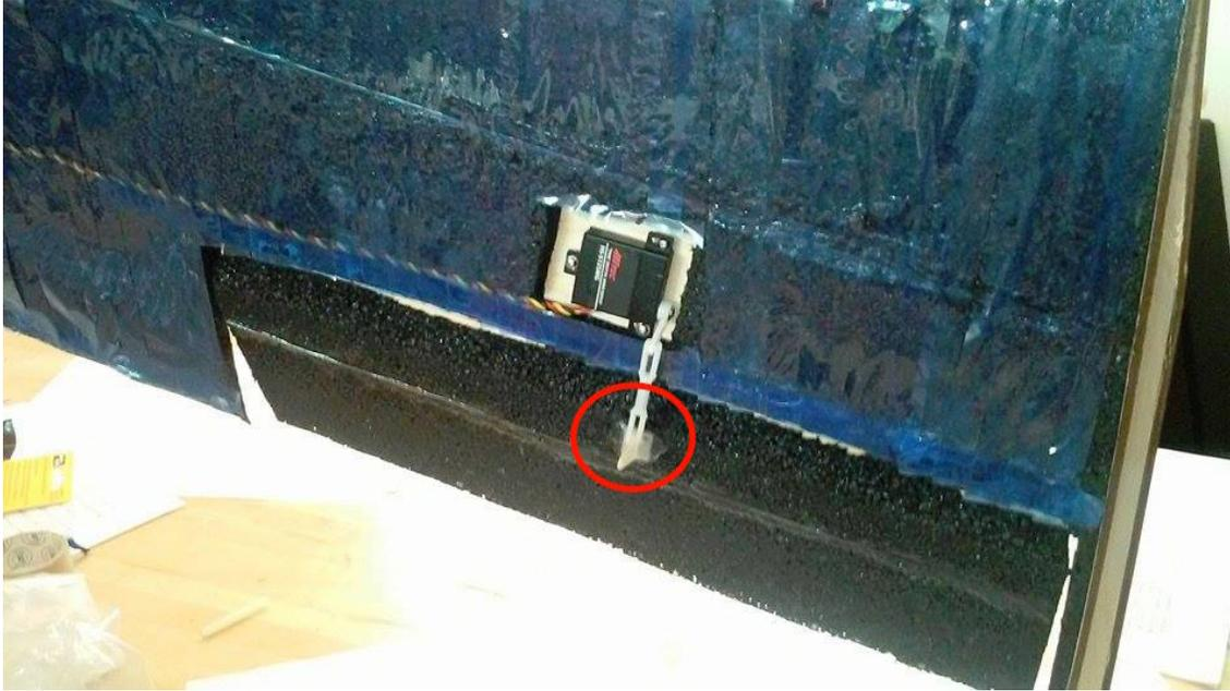
Figure 21: View of the bottom of the port side wing and elevon. Below the control arm (circled in red) is the carbon spar inserted into the elevon to give it some rigidity. To the left of the servo is the connection wires imbedded in a channel pulled out using plier and covered in tape.
