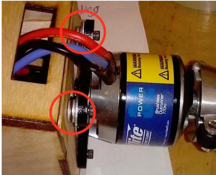
Figure 15: View of the motor attached to the front of the fuselage. Washers were added to the top bolts (circled in red) to tilt the motor down in order to align the thrust line to be parallel with the fuselage.
