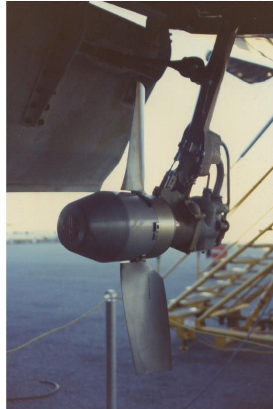
Ram air turbine: F-105 (Left) and Boeing 757 (Right)
