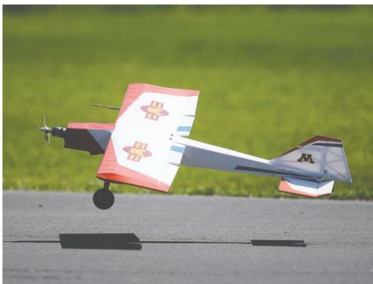
(a) Flight test vehicle on approach
