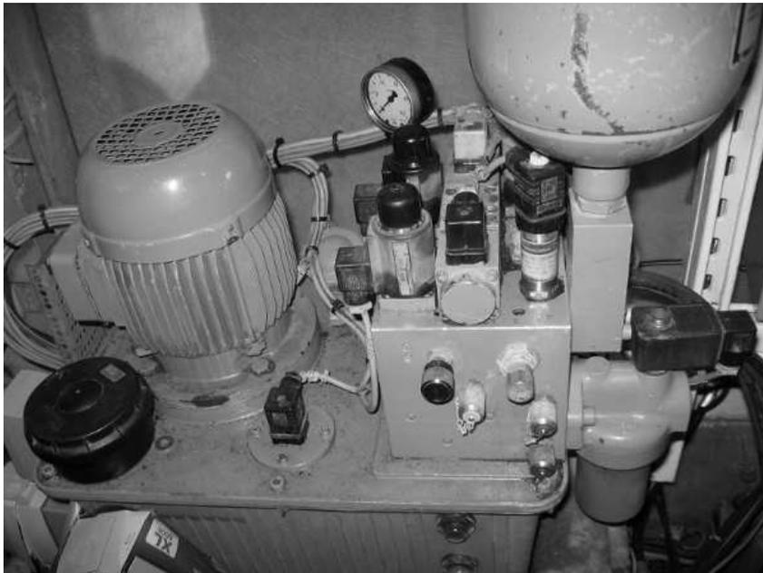
Figure A.2: The hydraulic motor in the nacelle.
