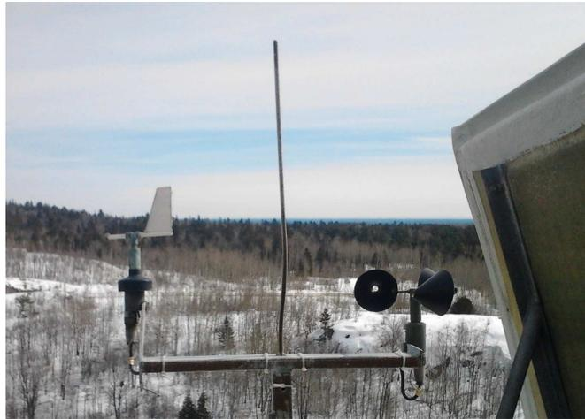
Figure 2.4: The anemometer and wind vane on the turbine nacelle.
