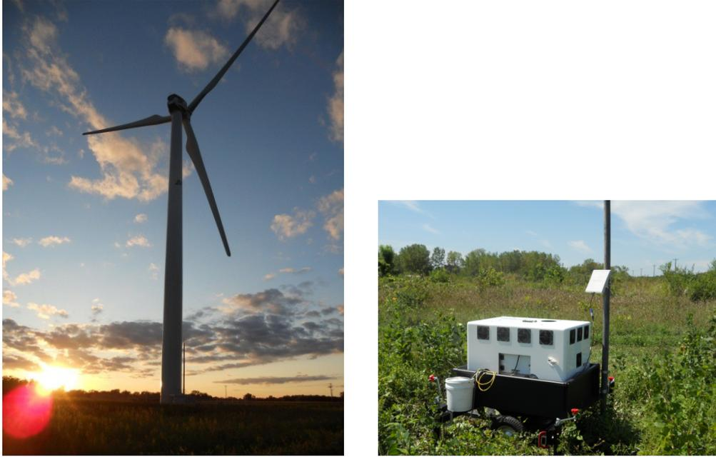
Figure 5.1: Clipper Wind Turbine located in UMore Park, Rosemount, MN (left). LIDAR used to measure wake profiles at various distances downstream (right)
