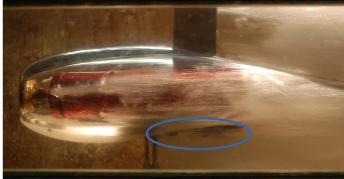
Figure 3.7: Photograph of the test vehicle from the bottom view. Lateral planing induced by the rotary shaft
