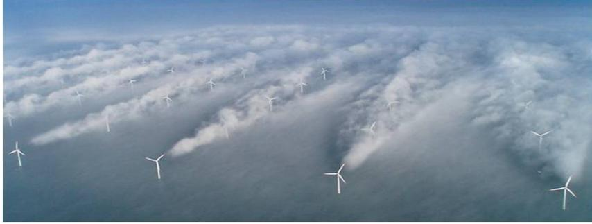
Figure 2.10: Aerodynamic interactions in the Horns Rev wind farm. Photo credits: Vattenfall Wind Power, Denmark.
