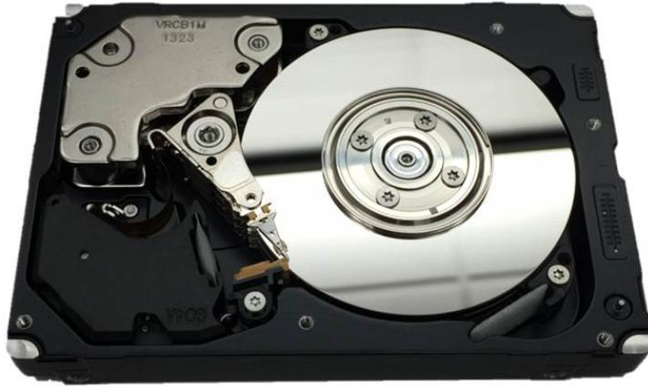
**Figure 2.1:** Picture of a hard disk drive with the front cover removed
