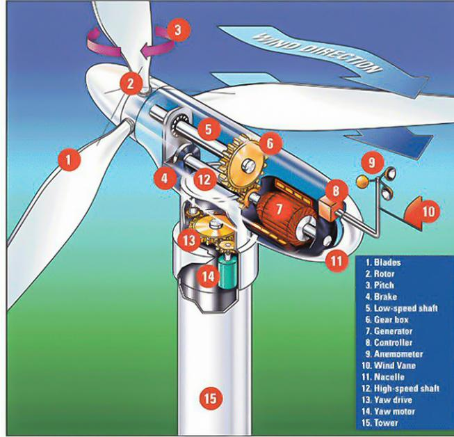
Figure 2.2: Wind turbine structure and components [3].
