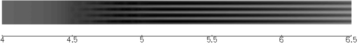
Figure 15. Snapshot of the flow from a simulation where the flow did not transition. Mach number is 2.9, Re = 635000/\text{inch} , roughness amplitude k = 0.005 .
