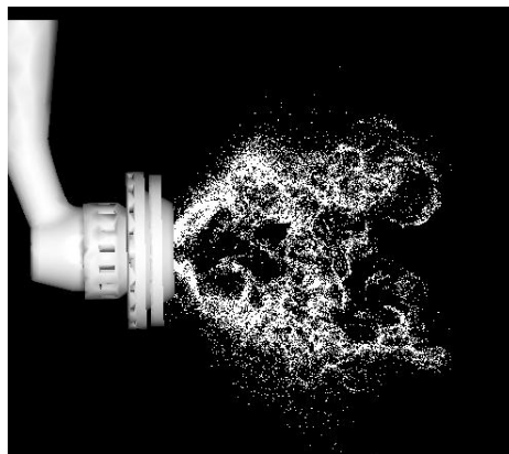
FIGURE 1. Snapshot spray from a gas-turbine fuel-injector.
