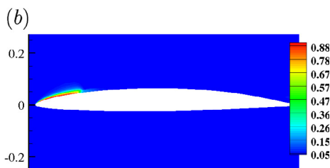
Fig. 9. (a) Comparison of pressure co-efficient ( C_p ) distribution to experiment, \circ : Shen and Dimotakis (1989), \Delta : Present. (b) Mean void fraction ( \bar{\alpha} ) contour for \sigma = 1.0 .
