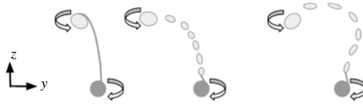
FIGURE 37. Schematic diagram showing blade trailing edge vortex sheet roll-up in the yz plane. The arrows show the sense of rotation of the vortices. The axial evolution is shown in the figure as we go from left to right.
