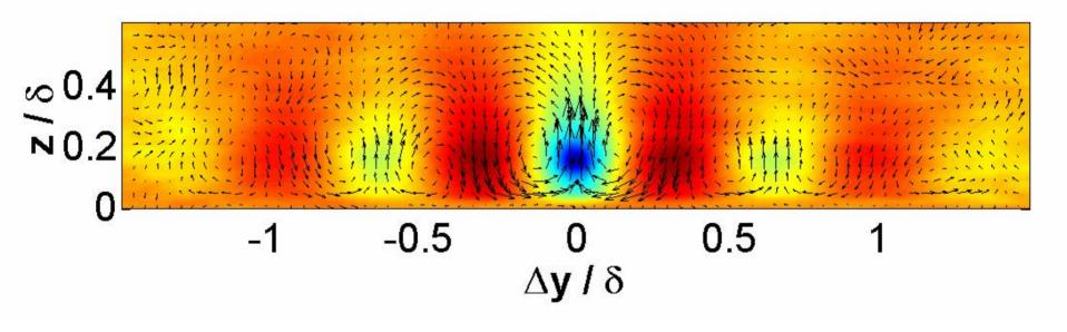
Conditioned on low-speed event at  $(0,z_{ref})$ , for the frames binned with  $0.5 < \lambda_z(u)/\delta < 0.75$
