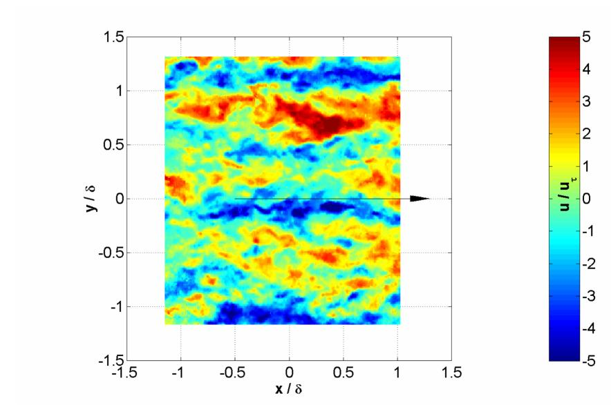
Establish a reference line, and bin frames according to dominant spanwise modes.
