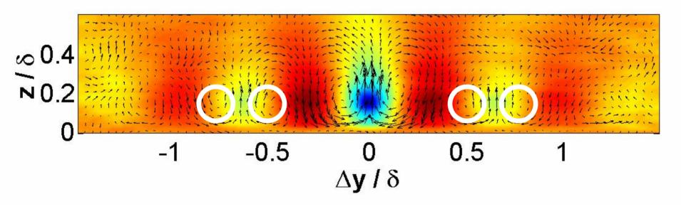
**Note**: the low-speed events are actually ejections (Q2), flanked by counter-rotating swirling motions
