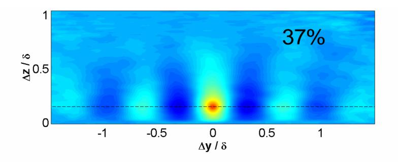
•Instantaneously the spanwise *u* behaviour seems to be well described by single spanwise sinusoidal modes extending a considerable distance in the wall-normal and streamwise directions.
