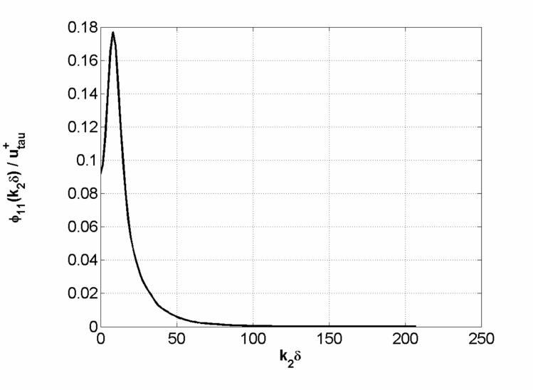
Energetic spanwise modes in the streamwise velocity signal at  $z_{ref} / \delta = 0.15$  ( $z_{ref}^+ = 140$ )
