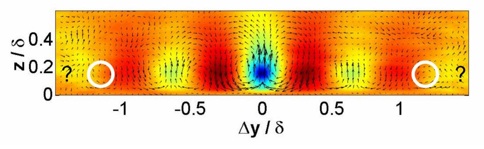
**Note**: the low-speed events are actually ejections (Q2), flanked by counter-rotating swirling motions
