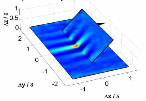
•Instantaneously the spanwise *u* behaviour seems to be well described by single spanwise sinusoidal modes extending a considerable distance in the wall-normal and streamwise directions.
