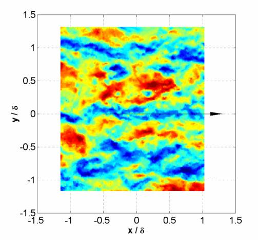
•Instantaneously the spanwise *u* behaviour seems to be well described by single spanwise sinusoidal modes extending a considerable distance in the wall-normal and streamwise directions.
