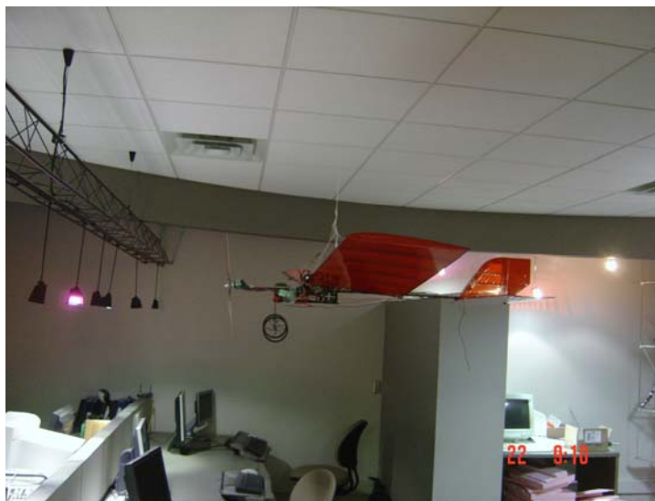
Figure 4. Pendulum swing to determine I_{xx} and I_{yy}
