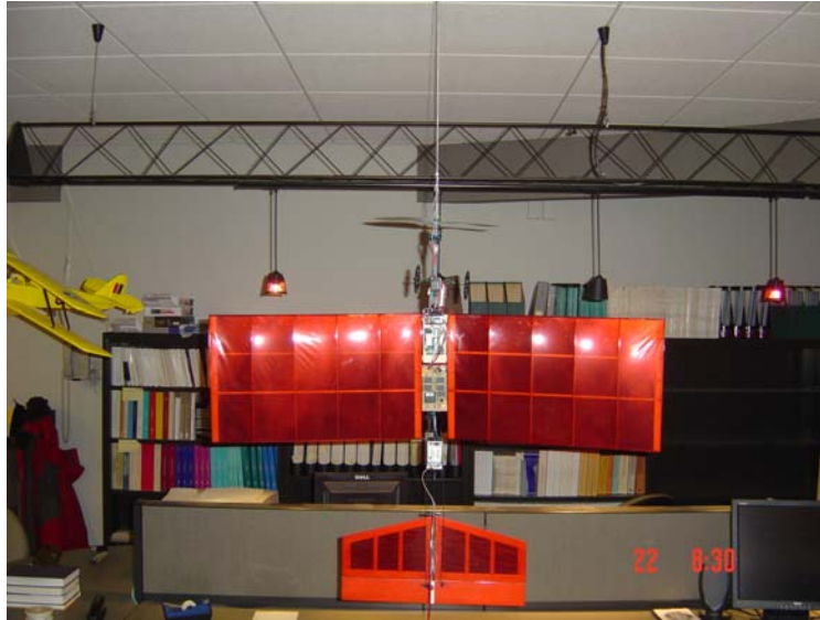
Figure 3. Pendulum swing to determine I_{zz}
